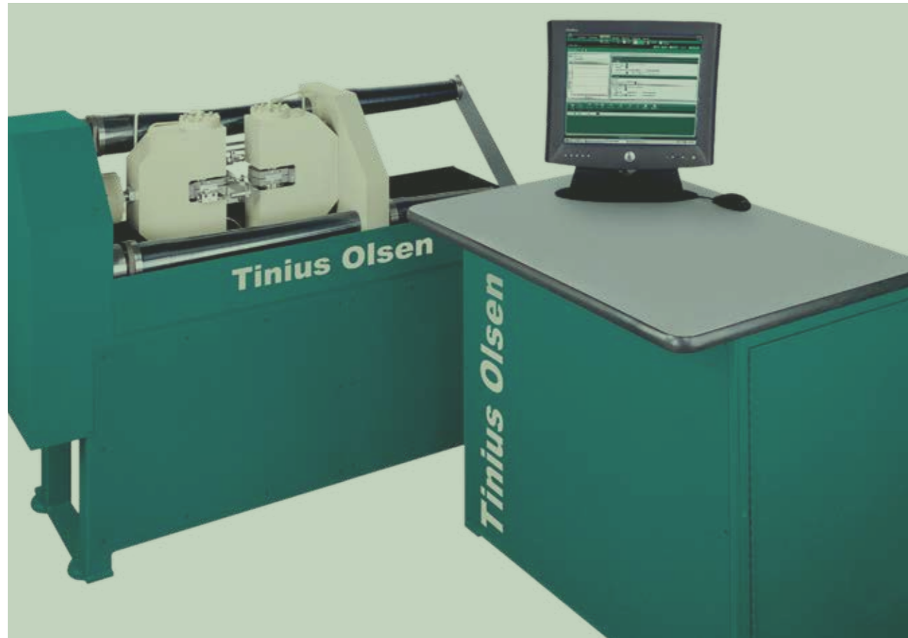
Basic 150kN capacity horizontal tensile testing machine, shown with Horizon software.
