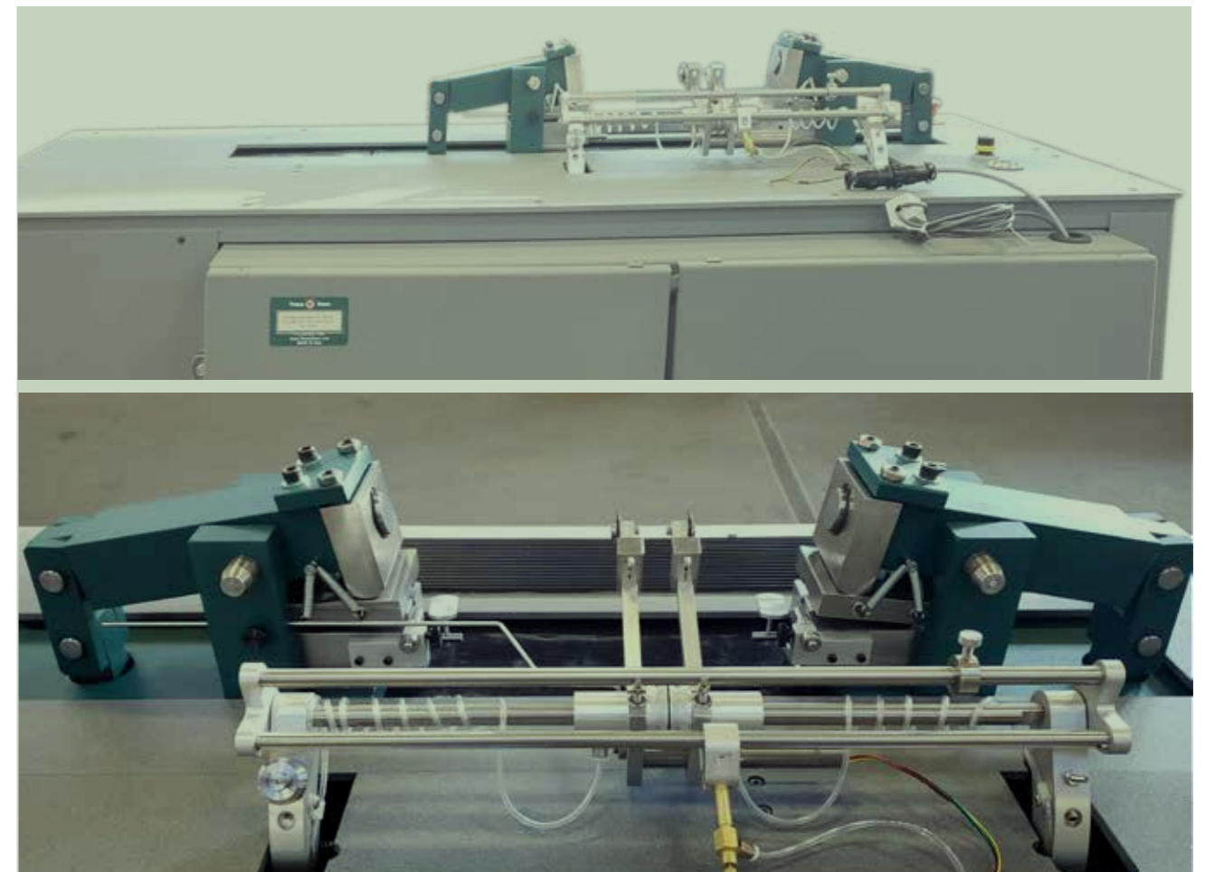
Basic 25kN capacity horizontal tensile testing machine, shown with optional extensometer.
